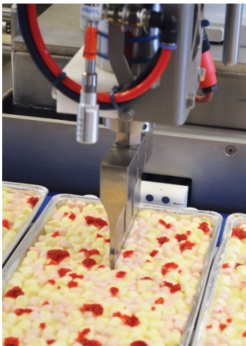
Picture 4: Once the tray is in position, the robot actuates the ultrasonic blade to portion the product based on the parameters entered on the HMI.
