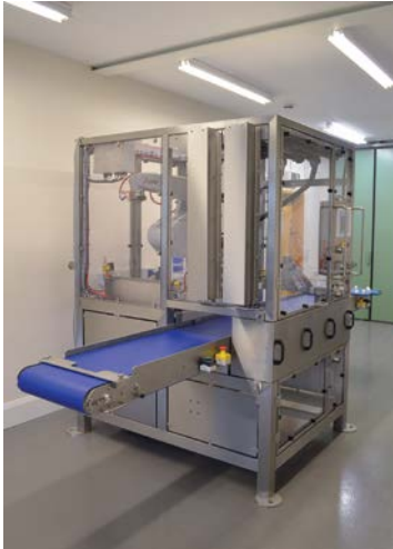
Picture 3: The solution offered by Mitsubishi Electric was built around an RF13 13kg payload, six axis robot, mounted within a stainless steel cell.
